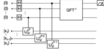
Figure 2: Phase estimation algorithm used to implement a quantum perceptron. The dot product of  $\vec{x}$  and  $\vec{w}$  is stored in the eigenvalue of the qubit state. Inverse QFT is used to extract the dot product ( $\phi$ ); the output becomes 1 if it is above the threshold and -1 otherwise. Figure taken from [16].
