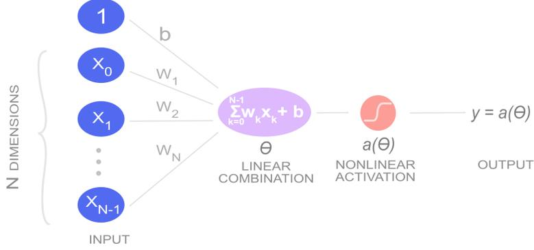
Figure 1: Schematic showing classical neuron. An  $N$ -dimensional input  $\vec{x}$  is linearly combined with an  $N$ -dimensional weight vector  $\vec{w}$  and a bias term  $b$ . The resulting dot product,  $\theta$ , is passed through an activation function to introduce a nonlinearity,  $a(\theta)$ , to produce the output,  $y$ .
