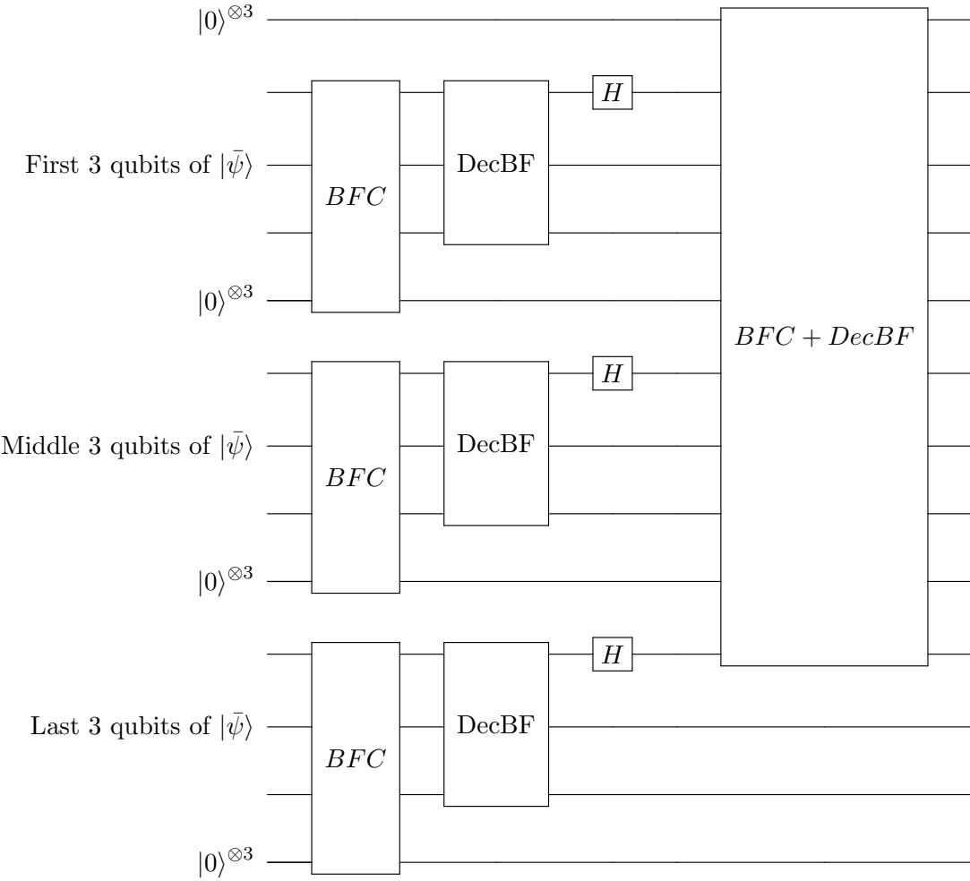
In the circuit above, “BFC” denotes Bit Flip Corrector for 3 qubits, described in Section 5.2. The first three BFC gates are applied to consecutive groups of three qubits. The last BFC and DecBF gate is applied to the second, sixth, and tenth wires shown in the circuit.
