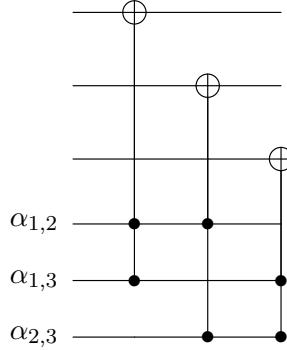
The two qubits indicated by the black dots have to be set to 1 in order for the target qubit to be flipped.
