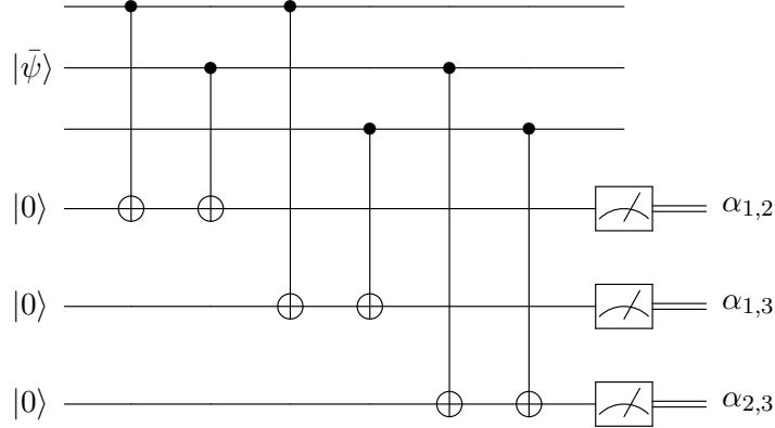
The measurement outcomes  $\alpha_{i,j} \in \{0, 1\}$  are called the syndrome of the circuit. The bit  $\alpha_{i,j}$  records the parity of the  $i$ 'th and  $j$ 'th qubits. If the qubits are equal (with respect to the standard basis), then  $\alpha_{i,j} = 0$ . Otherwise, it will be  $\alpha_{i,j} = 1$ .
